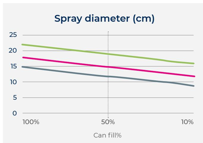
**i** All performance tests done with demineralized water – Spray diameter test done with a spraying distance of 15cm. Tests results are informative only and are non-binding.
